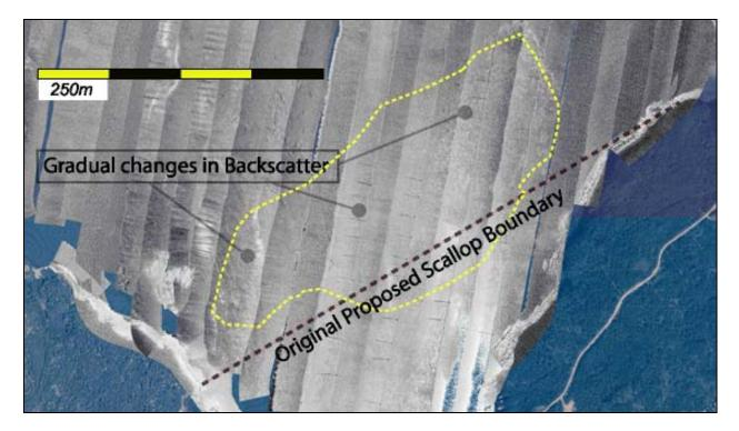
Figure 10: Detail of Knudsen sidescan data near the scallop zone boundary showing subtle changes in backscatter (background orthophoto SNB).
