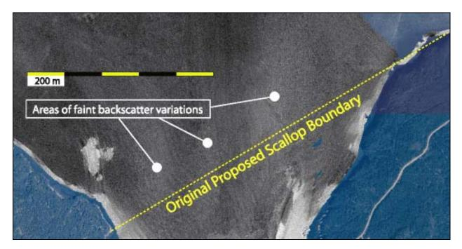
Figure 7: EM3000 backscatter of the scallop zone indicating subtle changes in the seabed sediment distribution (background orthophoto SNB).
