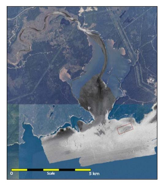
Figure 5: Overview of EM3000 coverage in the Musquash Estuary. Dark regions are low backscatter while lighter regions are high backscatter. Red box detail indicates location of images used in Figure 3. Note that the survey extent was limited to below the low water mark (background orthophoto SNB).
