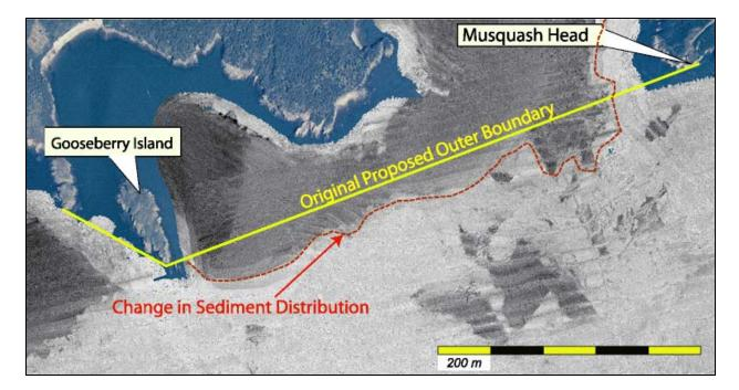
Figure 6: EM3000 backscatter image of the outer extent of Musquash Harbour showing the change in sediment distribution and the original proposed outer MPA boundary (background orthophoto SNB).
