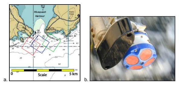
Figure 4: (a) Diamond pattern selected for the ADCP survey of the entrance to Musquash Estuary. Red = west diamond; Blue = central diamond; Green = east diamond (background CHS Chart #4128). (b) ADCP transducer (red, white & blue) mounted on pole on the *Mary-O*. The black transducer is downward-looking echosounder.
