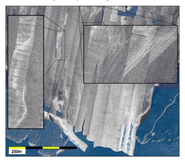
Figure 9: Two details of Knudsen sidescan data showing oceanographic fronts which appear in the image as linear striping of high backscatter (background orthophoto SNB).
