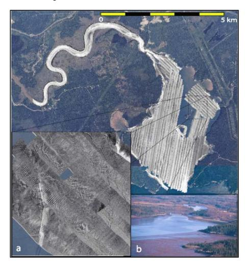
Figure 8: Overview of sidescan coverage in the Musquash Estuary. Detail (a) exemplifies results showing subaerial channels developed on the intertidal mudflats in less than 2 metres of water. Detail (b) presents a low-tide aerial view of the same locale (background orthophoto SNB).
