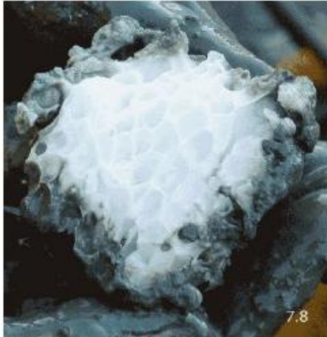
Figure 2: Methane hydrate obtained from the sea floor during a research expedition off the coast of Oregon (World ocean review)
