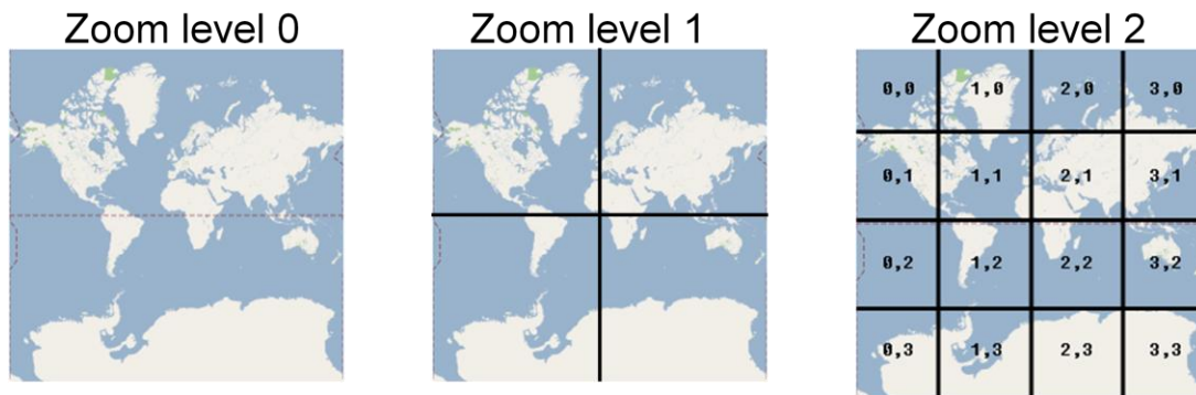
Figure 3.1 - Tile creation for Google Maps, each tile is subsequently divided into four new tiles. [Google Maps v2, 2010]
