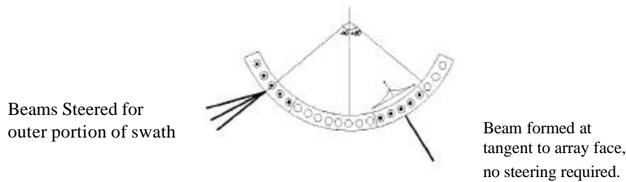
Figure 8: Illustration of the design of a curved array of elements in a multibeam sonar (Kammerer, personal communication).
