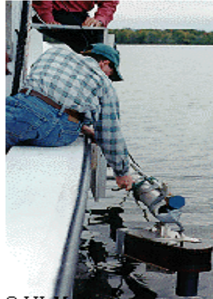
Figure 10: Securing the the Reson 9001 transducer to Mary O vessel, Burton bridge Hydro Field Camp (photo courtesy of J.V Martinez).
