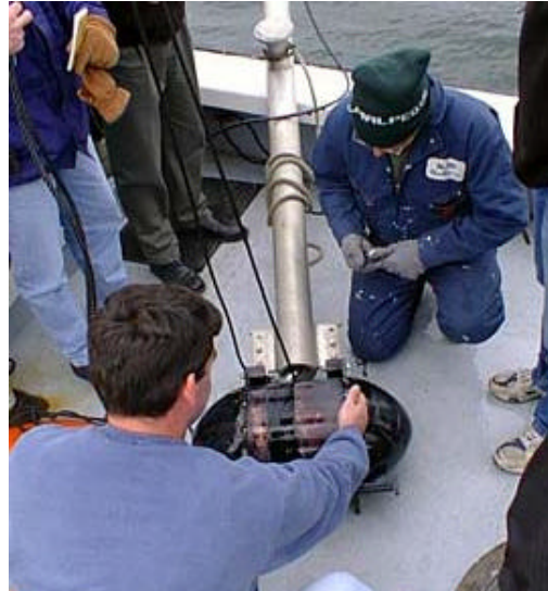
Figure 9: Attaching the Reson 8101 transducer to poll mount, St. Andrews Hydro Field Camp (photo courtesy of Dr. D. Wells).
