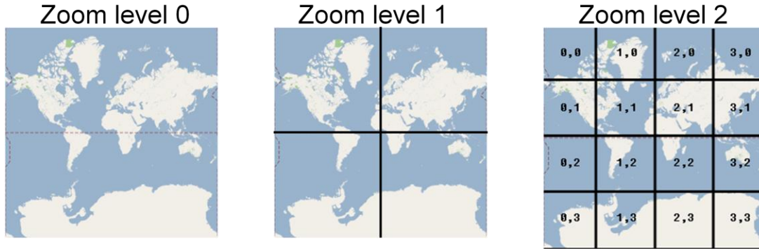
Figure 4. Tile creation for Google Maps, each tile was subsequently divided into four new tiles [Google Maps v2, 2010].
