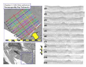
Beginning in may of 2002, the St. Andrews harbour and approaches survey was completed as an instrument test trial (see Hydrocamp results below). This repeated transit sections run by the Creed 10 years earlier providing higher resolution data on the linear trains of smaller pockmarks developed SE of Navy Island. This is a region where the highest density of pockmarks has been developed.
