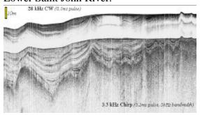
We use a standard 28 kHz source together with a single 3.5 kHz element. For lacustrine sediments we can achieve up to 15m penetration at 28 kHz and over 60m at 3.5 kHz.
