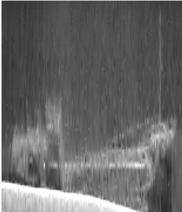
Figure 8: Compressed water column image of sunken wreck (80:1 compression ratio).
