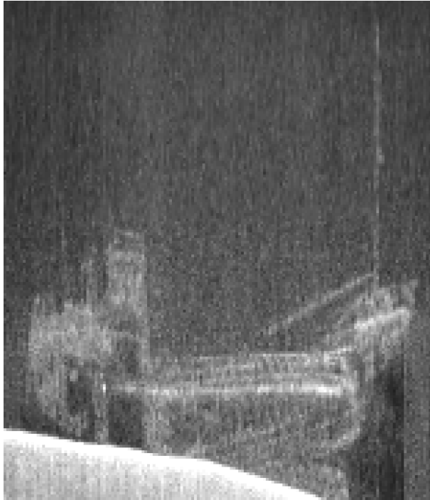
Figure 6: Compressed water column image of sunken wreck (20:1 compression ratio).
