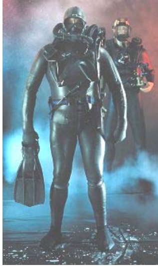
Figure 2-3 Diver suited up in CUMA2 Equipment, a mixed gas re-breather system for MCM Operations to a depth of ~80 metres. DND Photo.
