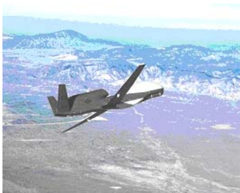
Figure 3-1 Global Hawk surveillance UAV is fitted with a range of electro-optical systems and can generate geo-spatially registered video mosaics in near real time. USAF Photo.
