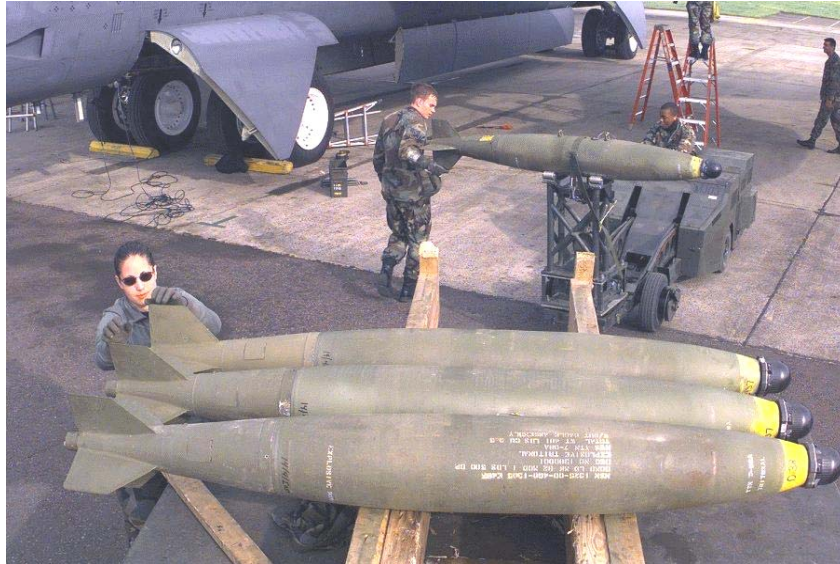
Figure 2-10 US Mk82 Bombs being loaded onto a B52 Bomber, a conversion of the nose arming mechanism changes this free fall bomb into the MK36 Destructor Sea Mine. (USAF Photo)
