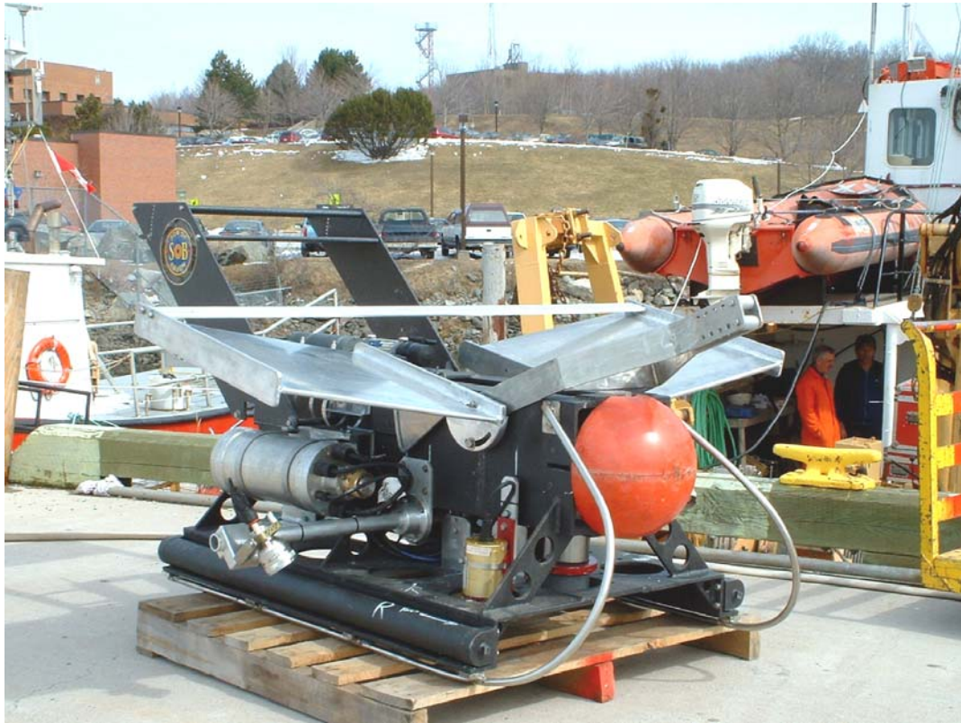
Figure 2-9 – TOWCAM II Vehicle fitted with video camera and digital still camera. (DFO Photo)
