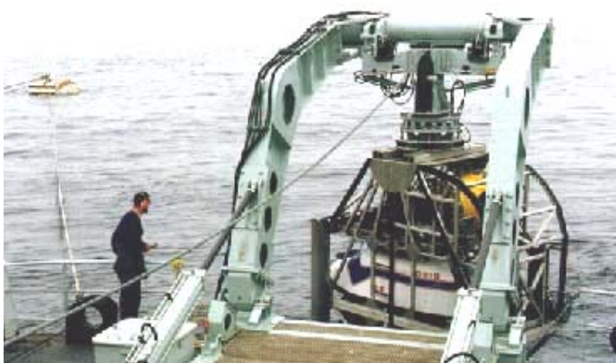
Figure 2-1 Deep Sea Intervention System (DSIS) ROV deployable to depths of 1400m DND Photo.
