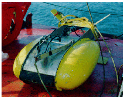
Figure 3.4: The housing casing of the Hunttec Deep-Towed Seismic System.
