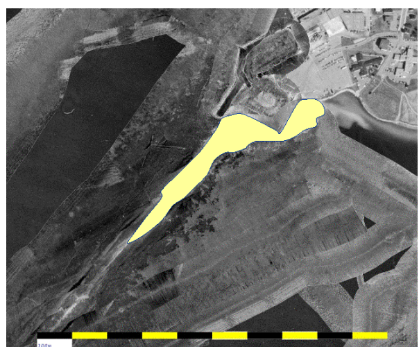
Figure 10. 200kHz with the high backscatter sediment plume highlighted.
