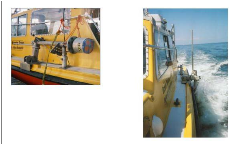
Figure 19. The pole mounted 600kHz Acoustic Doppler Current Profiler
