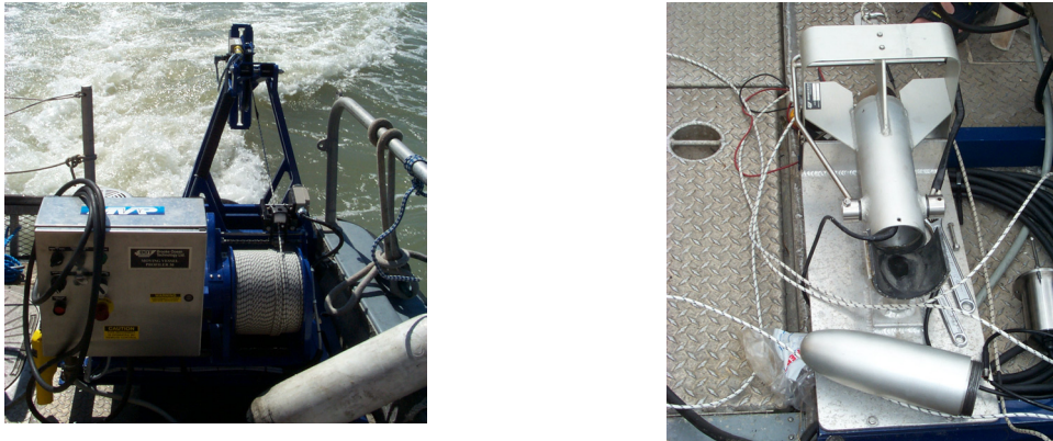
Figure 2 Moving Vessel Profiler 30 winch, overboarding sheave and freefall fish (disassembled)
