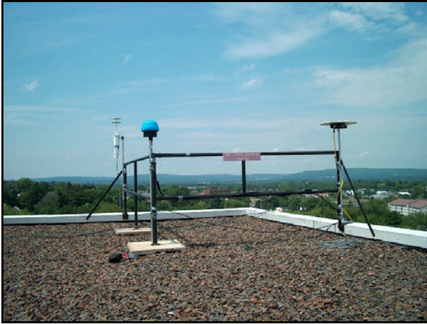
Figure 5: C-Nav mounted on Gillin Hall roof
