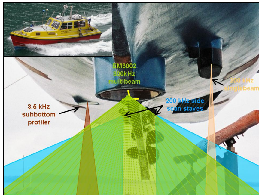
Figure 3.1 Hull of the CSL Heron with the transducer configuration.
