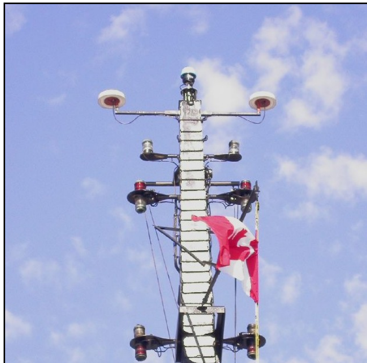
Figure 5.2: C-Nav and POS/MV Antennae Mounting Aboard Amundsen
