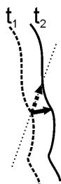
Figure 1.1 Illustration of over-estimate of crest displacement resulting from surveying a sand dune twice. The track line is the dotted line and the positions of the crest at times t_1 and t_2 are indicated. A better estimate based on tracking the morphology of the crest-line is represented by the solid arrow.
