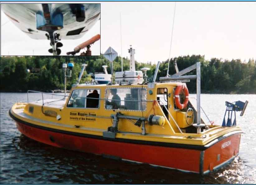
Figure 1: Above: The CSL Heron (length: 10 m). Inset: A view of the EM-3000 multibeam sonar.
