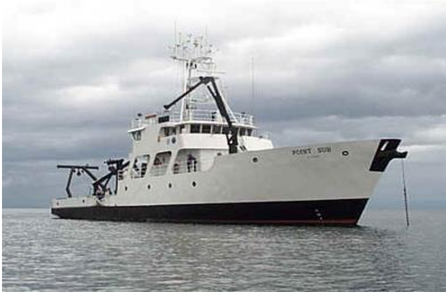
Figure 2. The R/V Point Sur was the survey platform for CONCORDE field operations. It is 135 feet in length with a beam of 32 feet and a draft of 9 feet.
